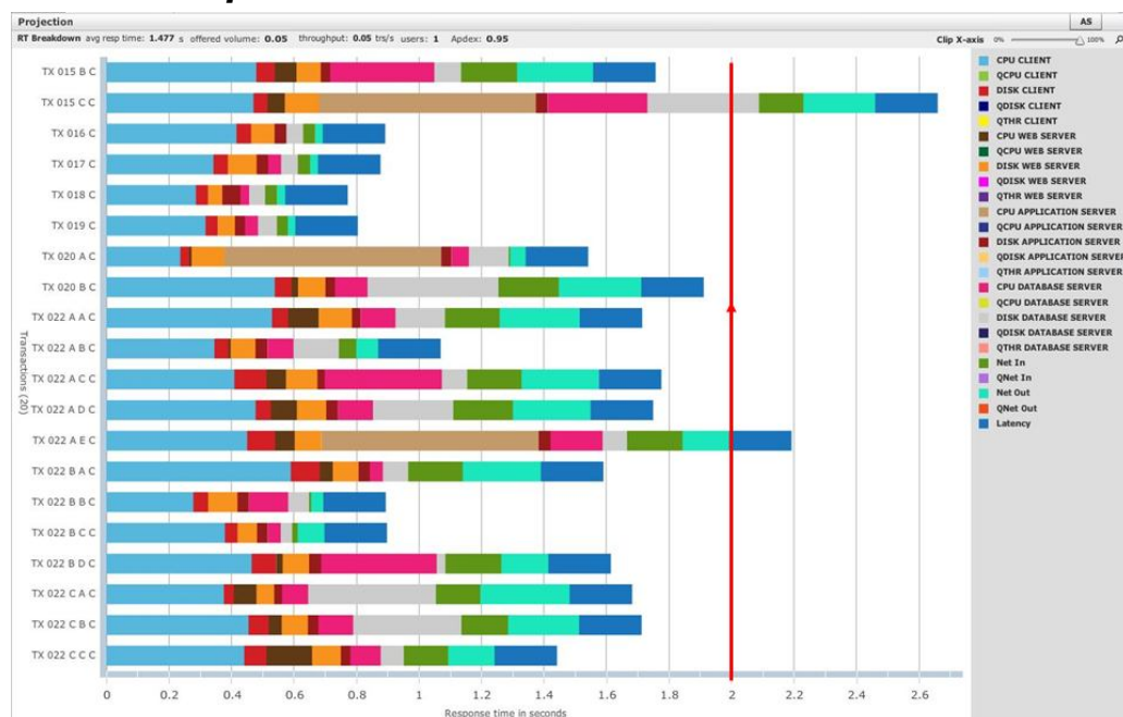
Figure 9. Two transactions still exceed the norm of 2 seconds. Nevertheless the application as whole scores an Apdex Index of 0.95, which is excellent.
